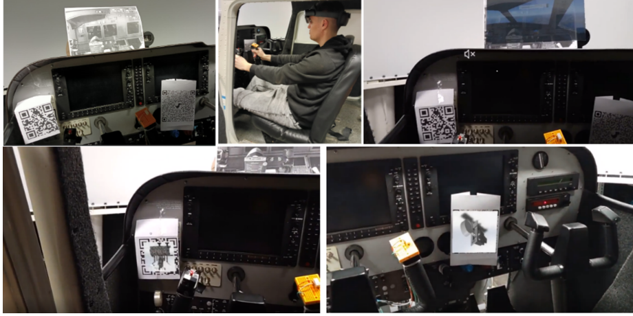
Fig. 8. Various stages of augmented reality marker integration in flight simulator training, showcasing different marker placements and sizes for enhanced cockpit interaction and tracking accuracy.
