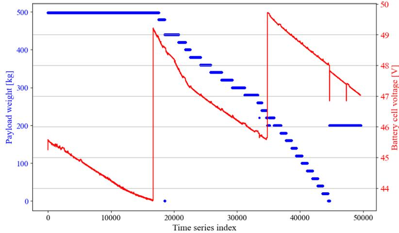
**Fig. 3.** Payload weight (blue) changes during test drives in October 2022. The test drives also included different levels of battery voltage (red), with two charges in between.
