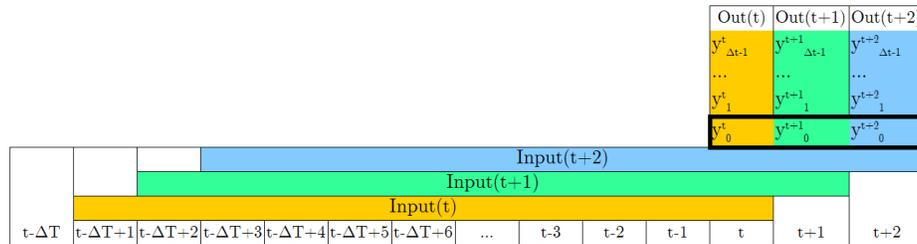
**Fig. 2.** Forecasting of MPC in time windows of a size  $\Delta T$  moving over an input time series  $X$ .  $\Delta t$  elements ahead are forecasted (forecast horizon). Only the first elements  $y_0$  of forecasts are taken to form an output sequence (elements in a bold frame).
