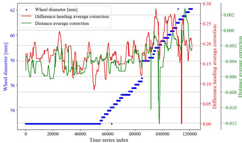
**Fig. 4.** Wheel diameter (blue) changes and resulting natural navigation correction values (red and green) during test drives in July and August 2023
