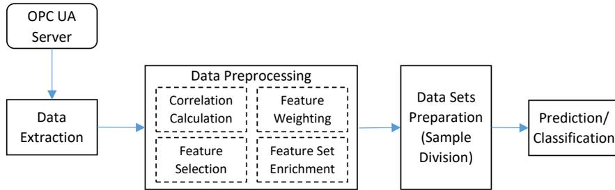
**Fig. 1.** Overview of the general methodology applied for predicting anomalies in the AGV operation.
