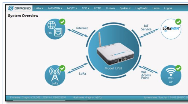
Fig. 3. LPS8 device configuration page after TTN connection.
